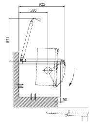
Cold Water inlet 1 (cleaning) FΙ Electrical inlet (power) Hot water inlet
